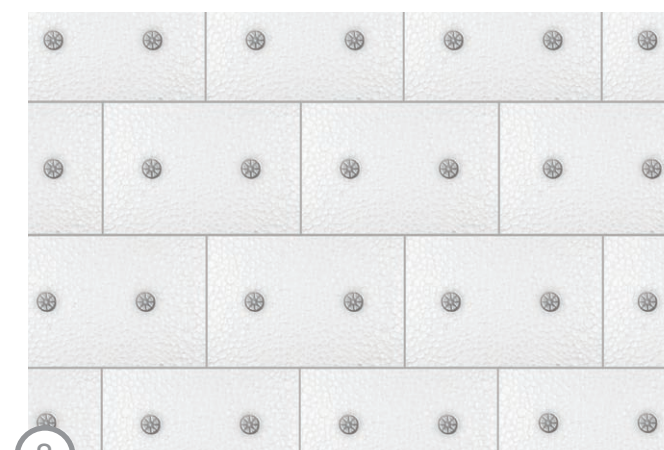
8 POLYSTYRENE – ANCHORS ARE PLACED CENTRALLY ON THE BOARD SURFACE
